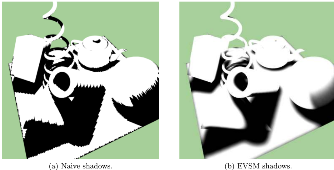
Figure B.2: Comparison of naive shadow mapping technique and EVSM with optimized 9x9 gaussian blur. Resolution of 256x256 depth map resolution.
